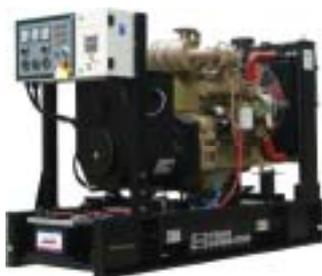
Cummins diesel engine made by DCEC China, Model:6LTAA8.9-G . With radiator at ambient temperature 40°C, fans are driven by belt, with safety guard, With DC 24V charge alternator.
