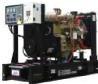
Cummins diesel engine made by DCEC China, Model:6BTA5.9-G . With radiator at ambient temperature 40°C, fans are driven by belt, with safety guard, With DC 24V charge alternator.
