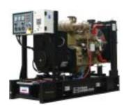
Cummins diesel engine made by DCEC China, Model:4BT3.9-G. With radiator at ambient temperature 40°C, fans are driven by belt, with safety guard, With DC 24V charge alternator.
